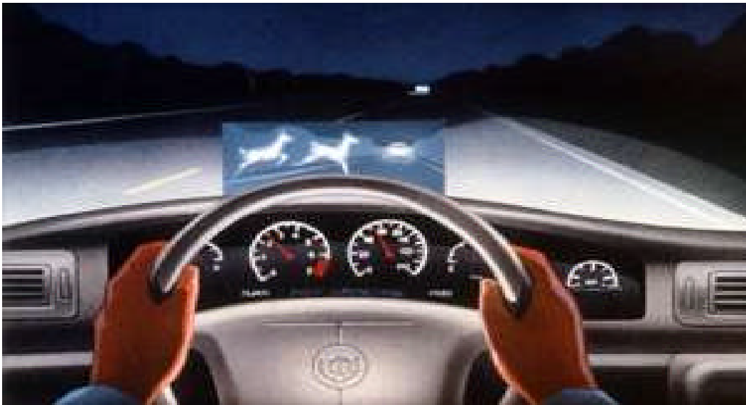
Photo 5: Cadillac DeVille night vision system (Illustration of the General Motors system from the GM Corporation website)
